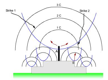
Figure 2: Illustration of lightning protection level design using the CVM.
