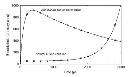
**Figure 5**: Comparison of a typical waveform obtained from a Marx-style generator with that observed in nature (e.g., Beasley et al 1982) from a progressing lightning downleader.
