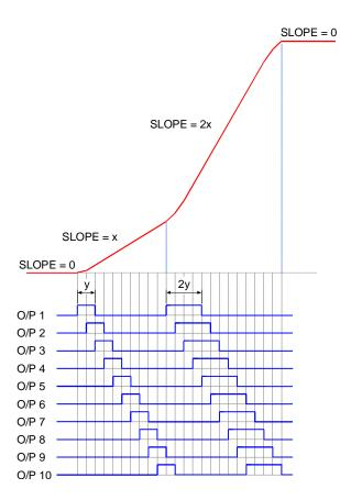
**Figure 6**: Simplified example of the "interleaving" principle of the HVAWG. The waveform slope is approximately proportional to the duty cycle.
