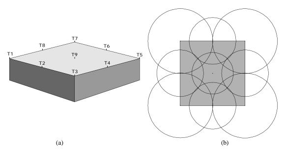
**Figure 3:** Example of the Collection Volume design method. Protection of a building 20 m high and 50 m wide and deep, using conventional finials 1 m high, 15 mm in diameter and with a tip radius of curvature of 1 mm. (a) 3D view. (b) Plan view.
