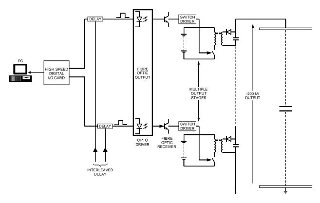
Figure 7: Schematic of the 150 kV prototype high voltage arbitrary waveform generator (HVAWG).
